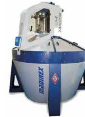
The Madirex granulating system eliminates all the restrictions of traditional systems. Depending on the grain size of incoming body -both for standard single-firing or porcelain stoneware obtained with MS-Drytech Porcelain technology - Madirex blends powder to obtain the ideal particles size distribution and moisture content.
